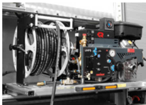
UHPS SKID - mounted in a fire truck
